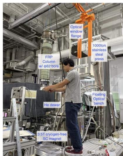
Fig. 1. Large-volume constant-load high-pressure device, equipped with high-NA optical access for ODMR experiments under multi-extreme conditions.
